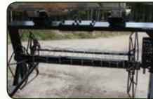
**Fence Torque** - Due to varying conditions of the fence prior to rolling, we've designed our RollMaster to withstand varying torque with a strong frame and pivoting hangers. During the rolling process you will have extra assurance that your fence will be wound up taunt for re-use.
