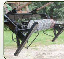
**All Types of Fence** - Whether you are removing strands of barbed or chain-link fence, you don't have to wrestle with a huge unmanageable monster of a roll any longer. Simply load the used fence onto the easy to use RollMaster quickly and safely.
