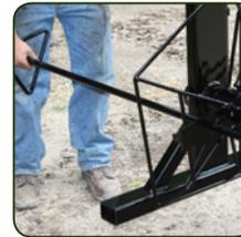
**Rolling** - The fence is rolled from a flat position, horizontal to the ground. Once the fence is secured to the steel bar, the hydraulic controls rewind the fence at variable speeds.
